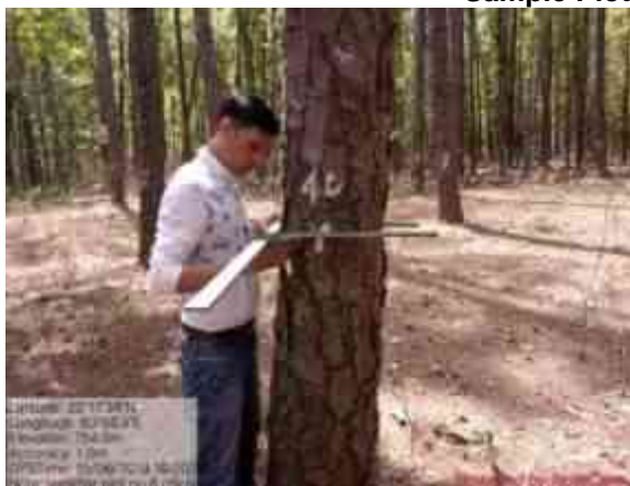
Diameter Measurement using Caliper
