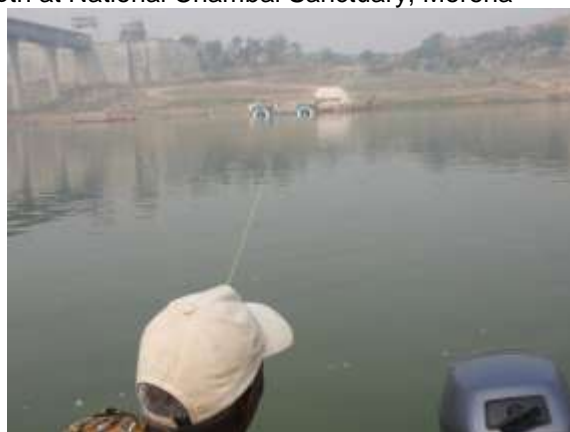
Measurement of various parameters across the river width at every 10 m distance, marked by red ribbon on synthetic rope
