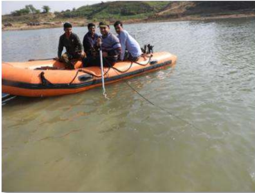
Data collection for river velocity from Parvati river, Sheopur, using Water flow Probe
