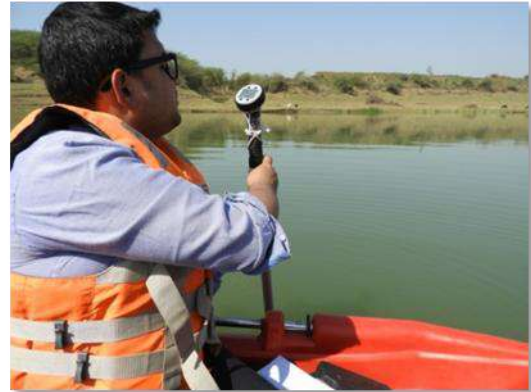
Data collection for river velocity from Parvati river, Sheopur, using Water flow Probe
